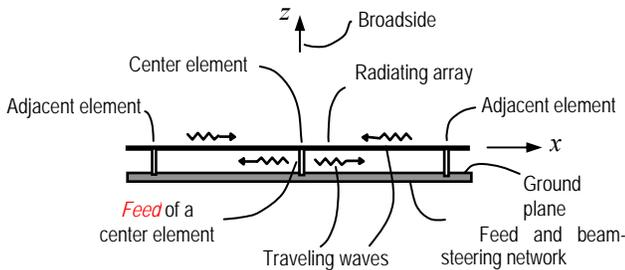
Fig. 3. Cross-sectional view around a center element of a TWAA.
