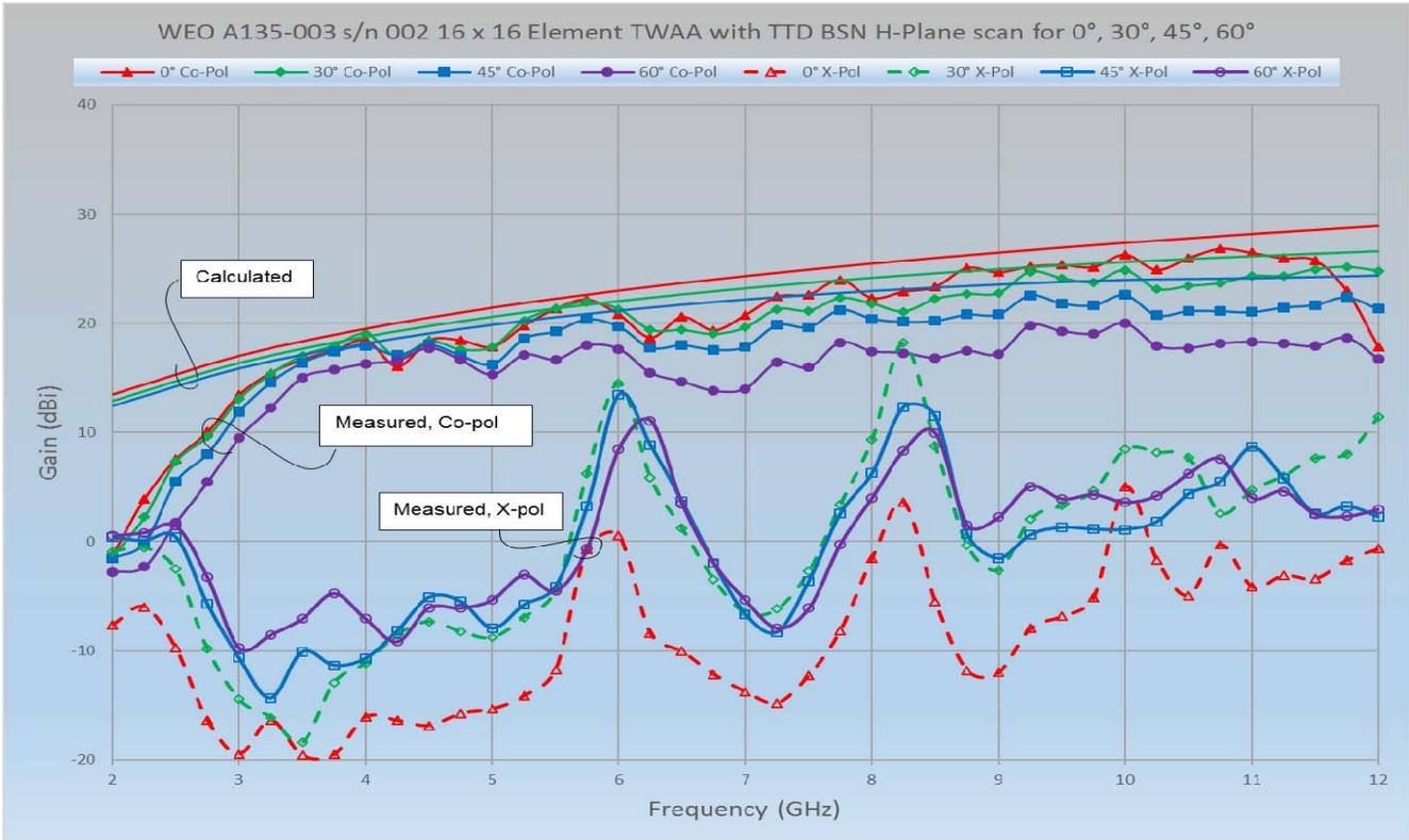
Fig. 5. Measured and calculated antenna co-polarization (Co-pol) and cross-polarization (X-pol) gain data over 2-12 GHz at scan angles of 0°, 30°, 45°, and 60° for *E*-plane scan (top) and *H*-plane scan (bottom).
