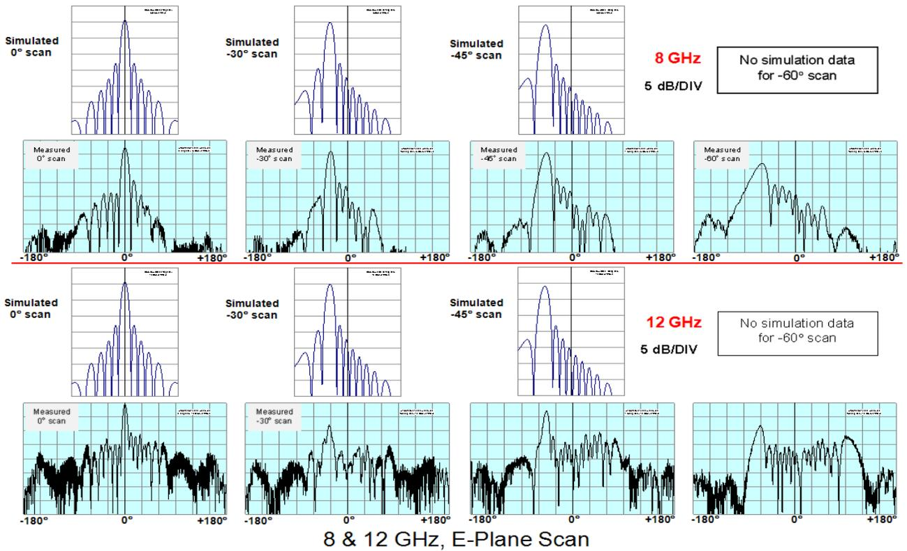
Fig. 6. Measured and simulated *E*-plane radiation patterns for *E*-Plane scan at 0°, -30°, -45° and -60° off broadside at 2, 4, 8, and 12 GHz.
