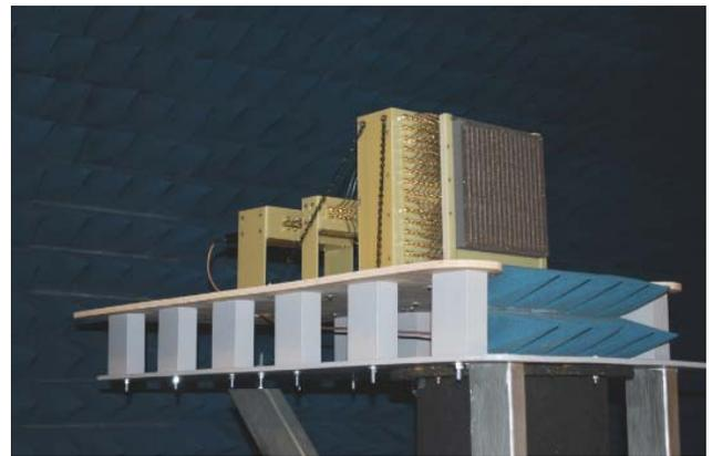
Fig. 4. A TWAA with three banks of TTD BSN being measured in WEO anechoic chamber.
