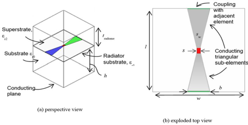
Fig. 2. (a) Unit cell of planar TWA array with planar bowtie dipole element, and (b) exploded top view of planar bowtie dipole element.
