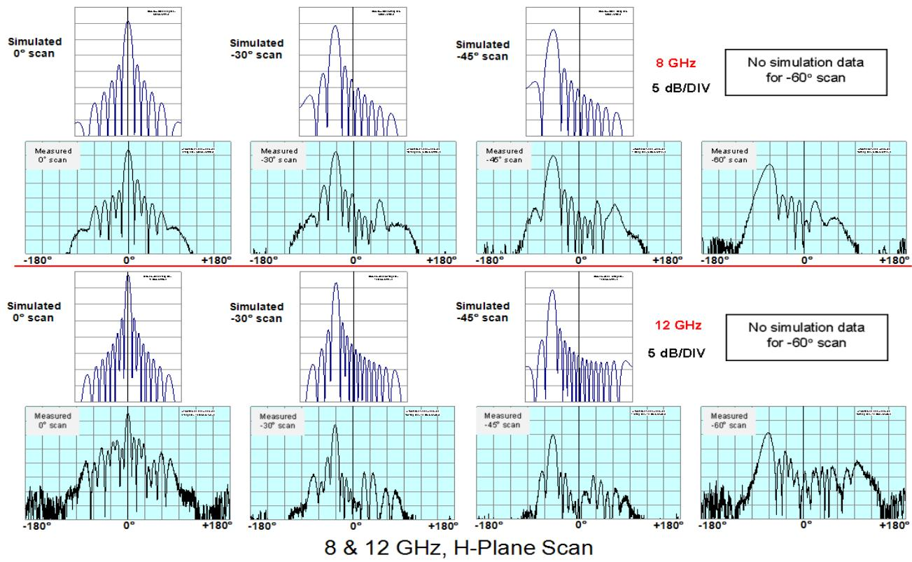
Fig. 7. Measured and simulated *H*-plane radiation patterns for *H*-Plane scan at  $0^\circ$ ,  $-30^\circ$ ,  $-45^\circ$  and  $-60^\circ$  off broadside at 2, 4, 8, and 12 GHz.
